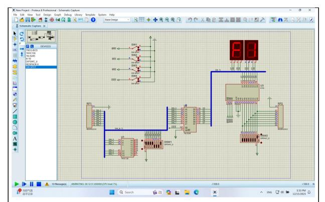
The operation mode of 6116 is determined by the combined effect of /WE, /0E, and /CE, all of which are active at low level.
