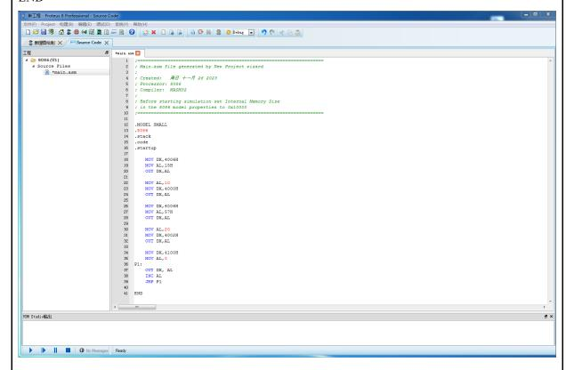
Experimental results: Through the programming and simulation operations of the above code, the initialization and control of 8253A were successfully achieved, but the DAC0832 failed to output various waveform signals.
